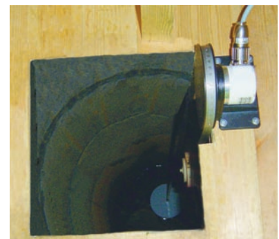
Vaisala Absolute Shaft Encoder QSE104 requires no backup battery to retain its position data
